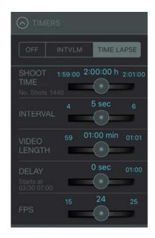
Time lapse is easily set up: based on a given shoot time (i.e. the total duration of the time lapse session) and the FPS (planned frames per second of the final edited time lapse video), Digital Director will automatically calculate:
