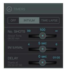
*Intervalometer* allows to select the number of shots the camera will take and the interval at which it will take them. The shoot time will be automatically calculated based on the number of shots and the interval selected.
